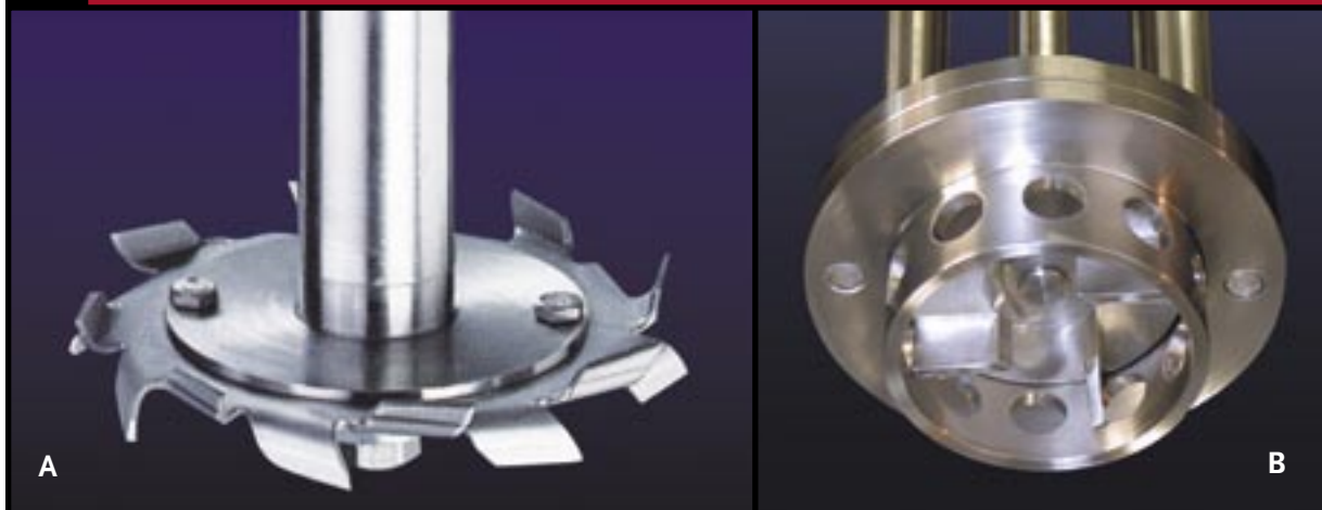
Figure 1. A high-speed disperser (A) is a good choice when moderate shear and high flow are needed, whereas a rotor/stator mixer (B) applies more intense shear than a disperser, but generates less flow.
